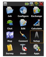
MAGNET Field not only controls the measurements of the instrument but also provides many COGO and adjustment calculations.
